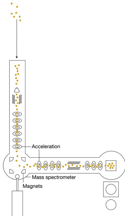
**How to produce nanoclusters:** A laser pulse heats a target and vaporizes some nanograms of material. The resulting plasma is cooled through both a helium gas pulse and expansion into the vacuum of a thermalization chamber. The atoms aggregate into clusters; the size distribution can be varied by setting different parameters. A mass spectrometer is used to select a cluster of a precise number of atoms from the distribution generated by the cluster source.
